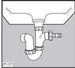
Push the drain hose onto the spigot and secure with a clip, ensure a loop is formed in the drain hose (see diagram) to prevent waste from the sink entering the washer-dryer.
